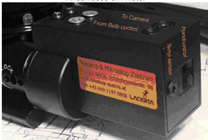
Anschlüsse am Motor
